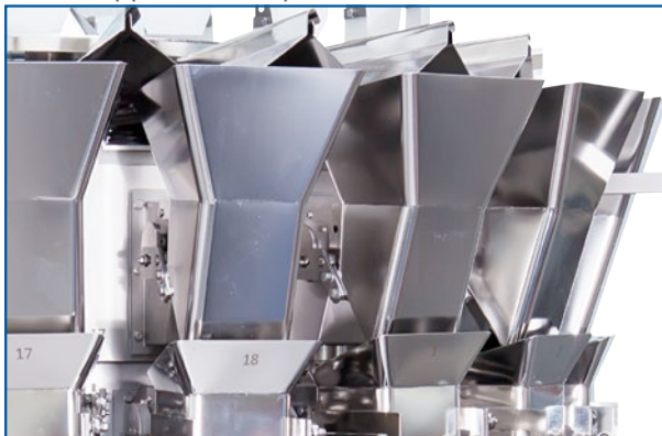
MultiWeigh® "Direct-Drive System", stepper motor operated hoppergates
